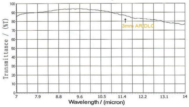
Ge windows with AR/DLC Coating of 3mm thickness
