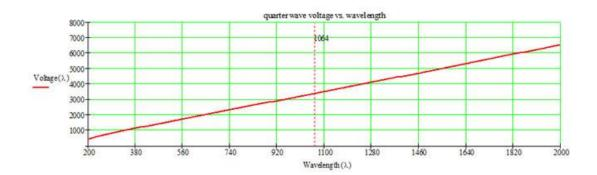
EO Q-Switch 1/4Wave Voltage Vs Vavelength (3x3x20mm)
